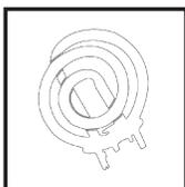
Heating Element (3). The 750-watt heating element provides the heat to boil the water in the boiling chamber.
