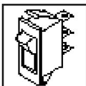
Cycle Start Switch (12). Pressing this switch will start the 210 minute distillation cycle.
