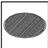
Filter (8). Before the distilled water flows into the drinking water container, it passes through an activated carbon filter pack to polish the taste of the water.
