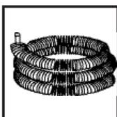
Condenser (6). A hollow, finned stainless steel tube where the steam from the boiling chamber is collected and cooled by the air from the fan. The steam is converted into high-purity drinking water. At the top portion of the condensing coil there are two small holes. These are two gas vents to allow volatile compounds to escape.
